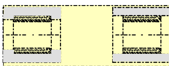
Ill. 6a: Chamber-shaped bushing Ill. 6b: Without chamber bushing
